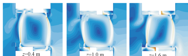
(c)调整出风口角度、回风口位置与风口尺寸
